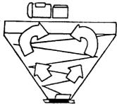
The unique vertical spiral mixing ribbon draws material from the bottom of the mixer and carries it up along the conical sides of the mixer body.
